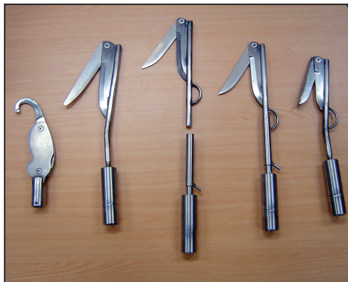
Figure 3.4 A range of disentanglement tools for mounting on a pole. (Courtesy of the Australian Large Whale Disentanglement Response Network.)
