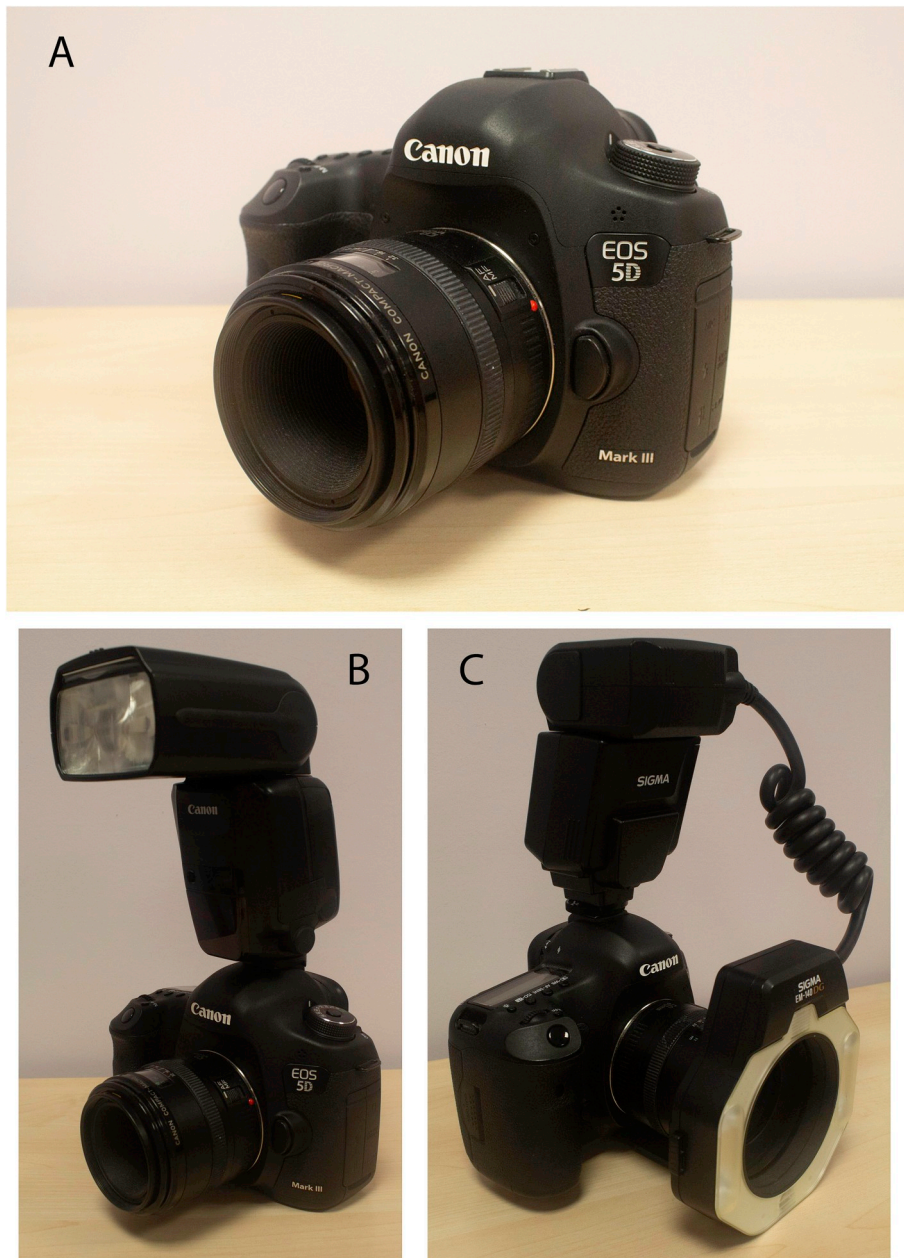
Fig. 1. Equipment used. (A) Canon EOS 5D mark III camera body with Canon EF 50mm f/2.5 Compact Macro Lens. (B) Canon Speedlite 600EX-RT Flash Gun. (C) Sigma EM-140DG Ring Flash (with 52mm adapter ring on lens).
